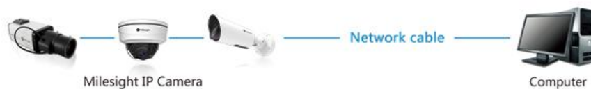
Figure 2-1-1 Connect the camera to the PC directly
